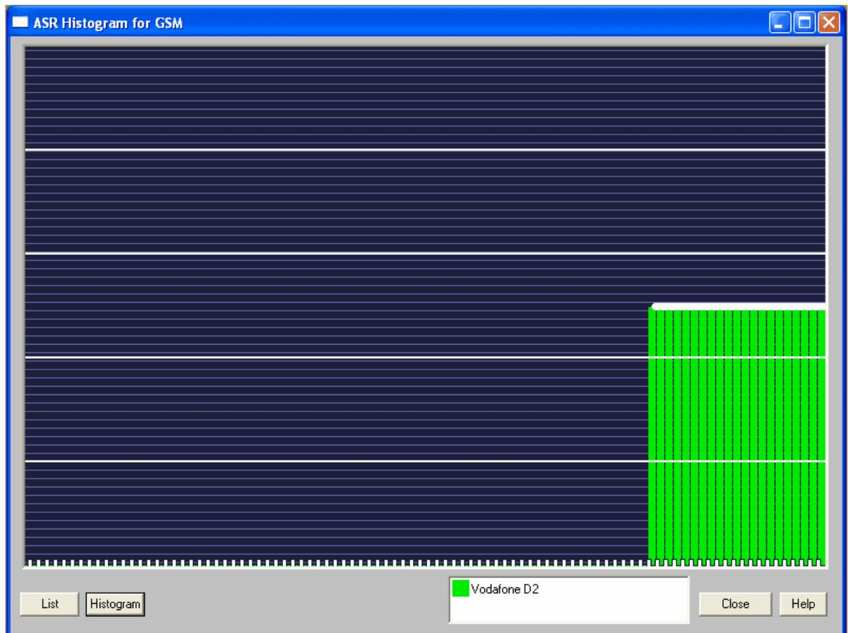
As you can see, the available providers each have it's own colour, and using the provider legend the providers can be identified (in this example, Vodafone D2 is green). The four white markers running through the display represent (from the bottom) 20%, 40%, 60%, 80% and the very top being 100%. The time scale is the total time as set on the [System State](#) page, using the option
