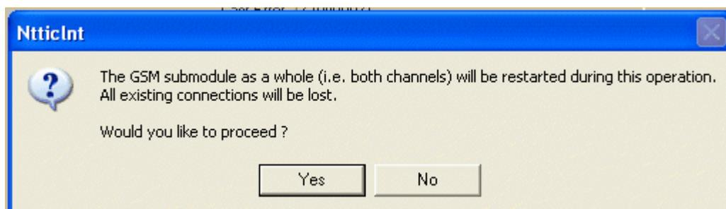
To reset the GSM interface, confirm this dialog and the interface will be reset
