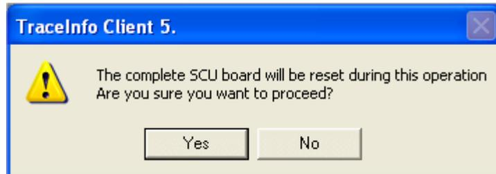
If you choose **Yes**, then the **complete** SCU board will be reset. **All** four interfaces will receive a reset signal, and any clients currently connected to these SCU interfaces will be cut off. You may choose **No** to abort resetting.
