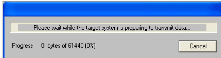
Dependent on the connection speed to the target system, this may take up to 30 seconds, then the trace information is buffered in the memory of the local machine
