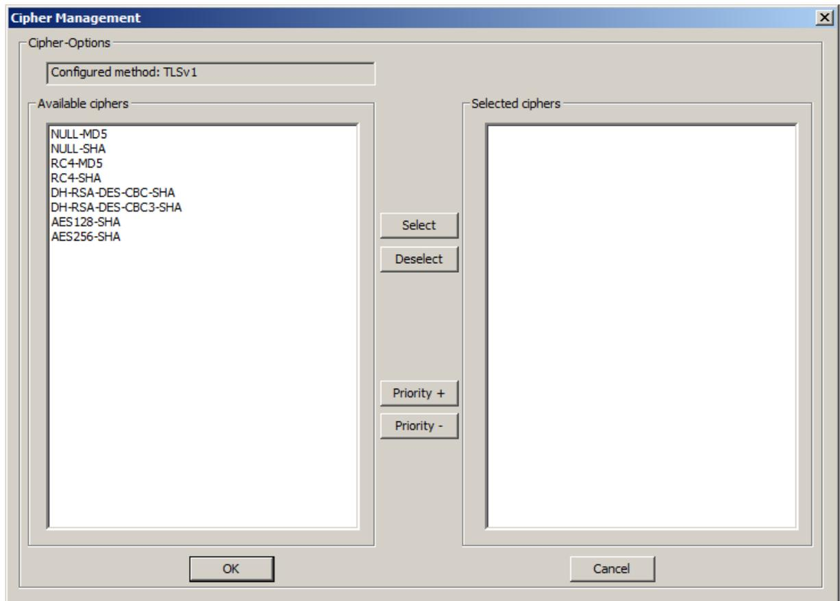
If none of the available ciphers is listed in the right window and you decide not to select at minimum one of the available ciphers in the left window, i.e. the right window remains empty, the system determines itself the "best" cipher respectively the most secure and compatible cipher during communication setup.
