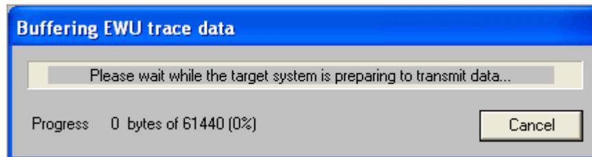
Dependent on the connection speed to the target system, this may take up to 30 seconds, then the trace information is buffered in the memory of the local machine. Then a dialog will appear, asking for a directory and filename for the EWU trace. It is advisable to save the EWU trace information in the same directory as the normal trace files. Once the file has been saved successfully, it can be viewed using the [Files](#) page
