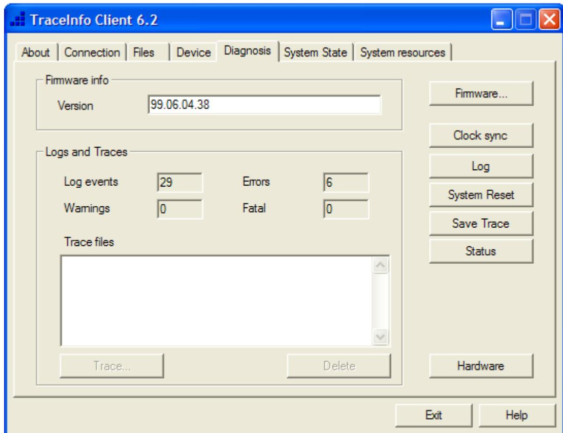
This page is the main point to download [traces and log books](#) from the target system. You also have the opportunity to upload new firmware to the target system, and carry out various maintenance tasks on the system.
